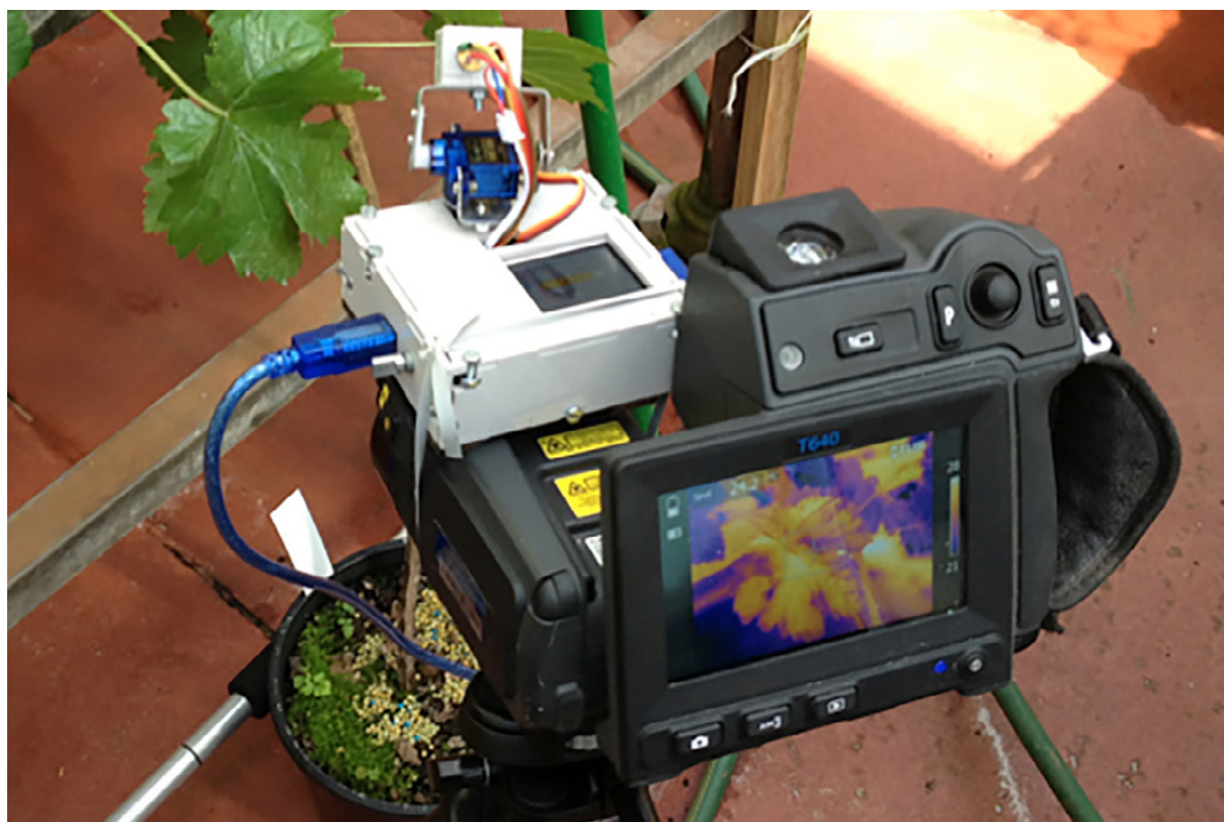
An infrared scanner, moved by two servo motors and controlled by an Arduino® Uno board, sits on top of a Forward Looking Infrared Camera to compare their respective performance (Sigfredo Fuentes).
